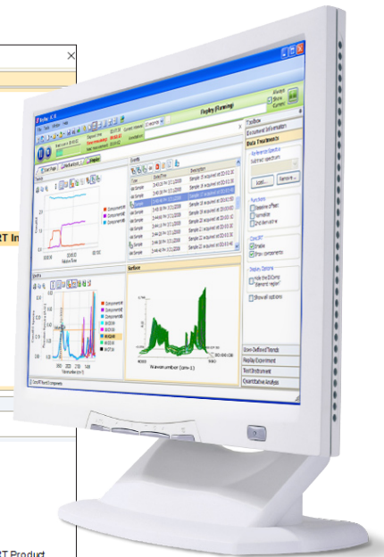
Left: The automatically calculated pure component spectra of a transient intermediate is shown above the ConciRT™ LIVE generated concentration profiles for the reaction
