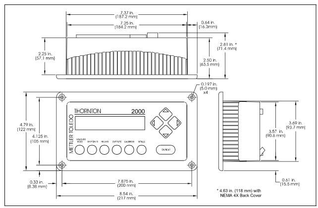
Figure 14.2a: Panel Mounting Dimensions
