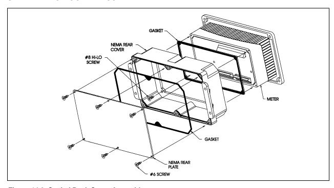
Figure 14.6: Sealed Back Cover Assembly
