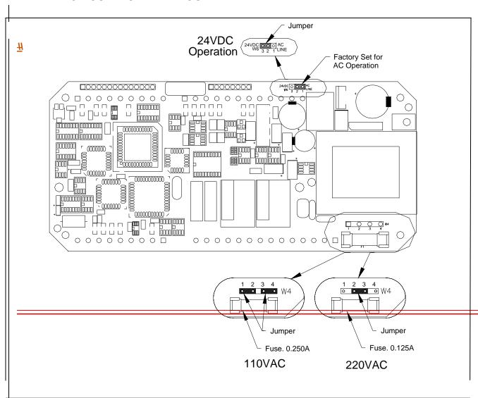
Figure 14.7: Printed Circuit Board Layout
