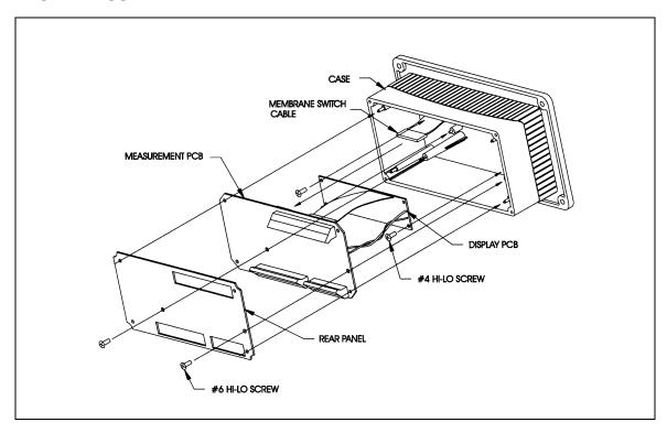
Figure 14.4: Exploded Assembly
