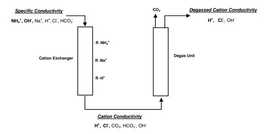
Fig. 4.2: Sample conditioning for specific, cation and degassed cation conductivity measurements used to calculate pH, CO₂ and anion concentration on power plant cycle chemistry samples
