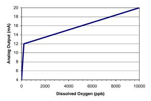
Figure 7.1: Bi-Linear Output Scaling
