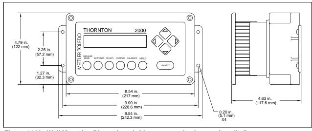
Figure 14.2b: Wall Mounting Dimensions (with accessory back cover installed)
