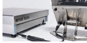
Terminals with IDNet interface can be ACC409xx adapter.
