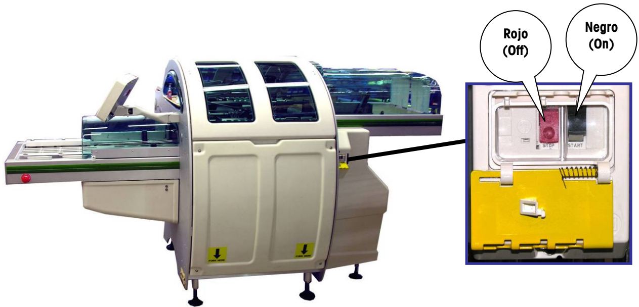
Interruptor de corriente principal
